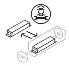
Replaceable control gear by an end-user
